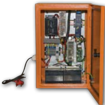
12Vdc / 4.5A with a 7Amps charger
